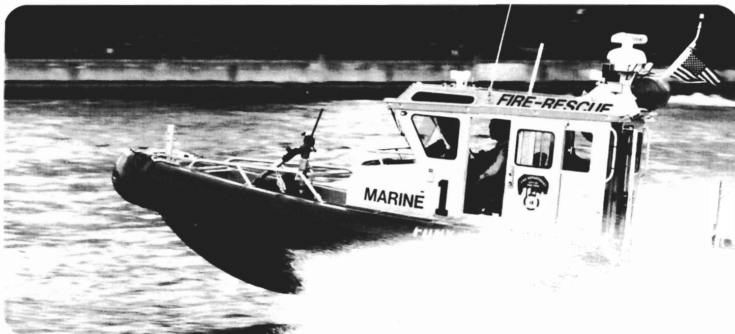
Fireboat Marine 1 Alpha makes its way through the Hudson River. The boat is 27 feet long, has the ability to travel up to 45 miles per hour and can transport 16 people. Although it is equipped for fire suppression, its design makes the boat ideal for water rescues.
